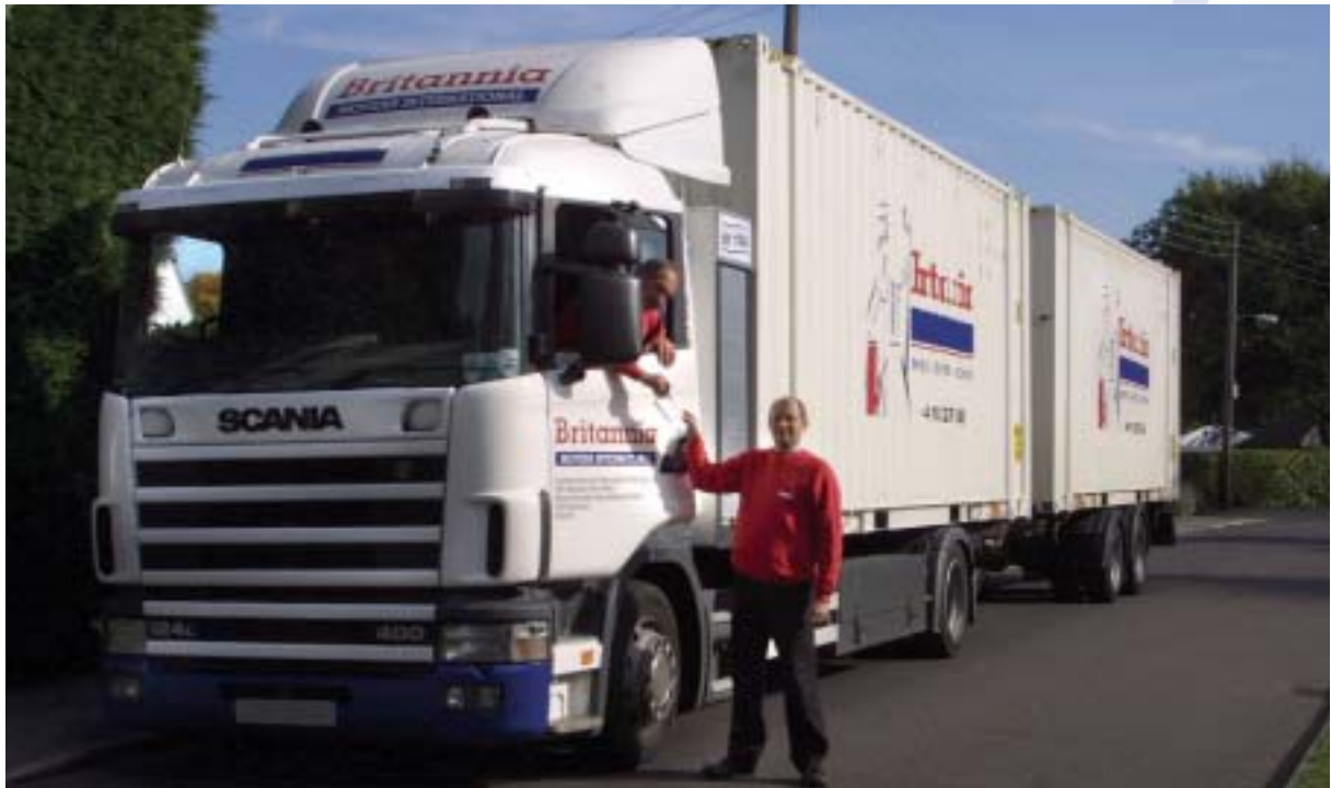
18m long, 4m high, 2.5m wide demountable bodied roadtrain capacity 96m 3 .
